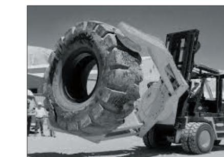
Hydraulic tire remover (rim flange push type) in operation
